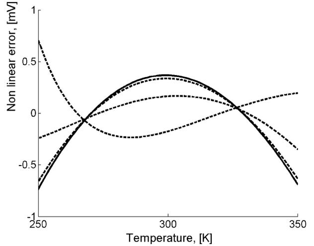
Fig. 3. The non linear error as a function of the temperature for a constant collector current (solid line) and for different PTAT/R collector currents (dashed lines; the TC of the resistor varies from  $5000$  up to  $10,000$  ppm/K); the Meijer parameter  $\eta_M$  has been considered equal to 3.
