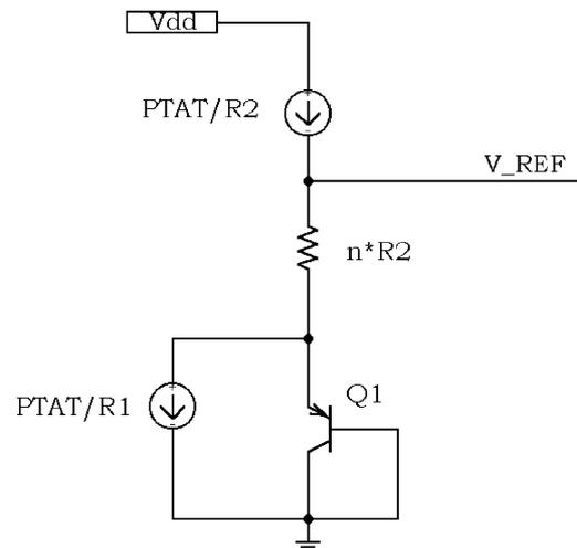
Fig. 6. Bandgap reference circuit for the implementation of an anti-shunt virtual resistor.
