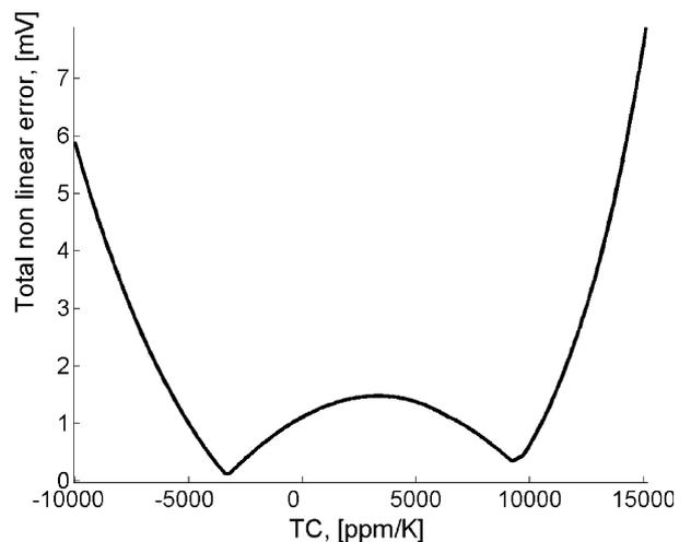
Fig. 4. The total non linear error (in the temperature range  $[250, 350$  K]) as a function of the TC of the resistor used to generate the PTAT/R collector current; the Meijer parameter  $\eta_M$  has been considered equal to 3.
