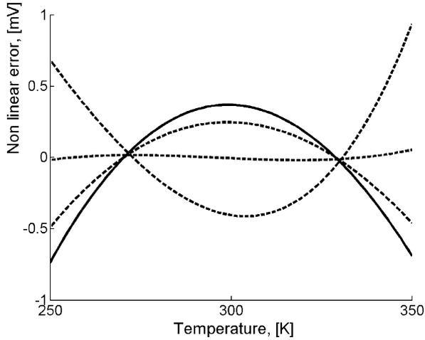
Fig. 1. The non linear error as a function of the temperature for a constant collector current (solid line) and for different PTAT/R collector currents (dashed lines; the TC of the resistor varies from  $-5000$  up to  $0$  ppm/K); the Meijer parameter  $\eta_M$  has been considered equal to 3.
