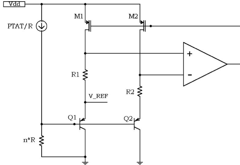
Fig. 5. Bandgap reference circuit for the implementation of an anti-series virtual resistor.
