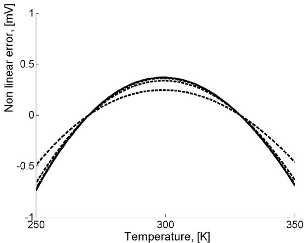
Fig. 2. The non linear error as a function of the temperature for a constant collector current (solid line) and for different PTAT/R collector currents (dashed lines; the TC of the resistor varies from  $0$  up to  $5000$  ppm/K); the Meijer parameter  $\eta_M$  has been considered equal to 3.
